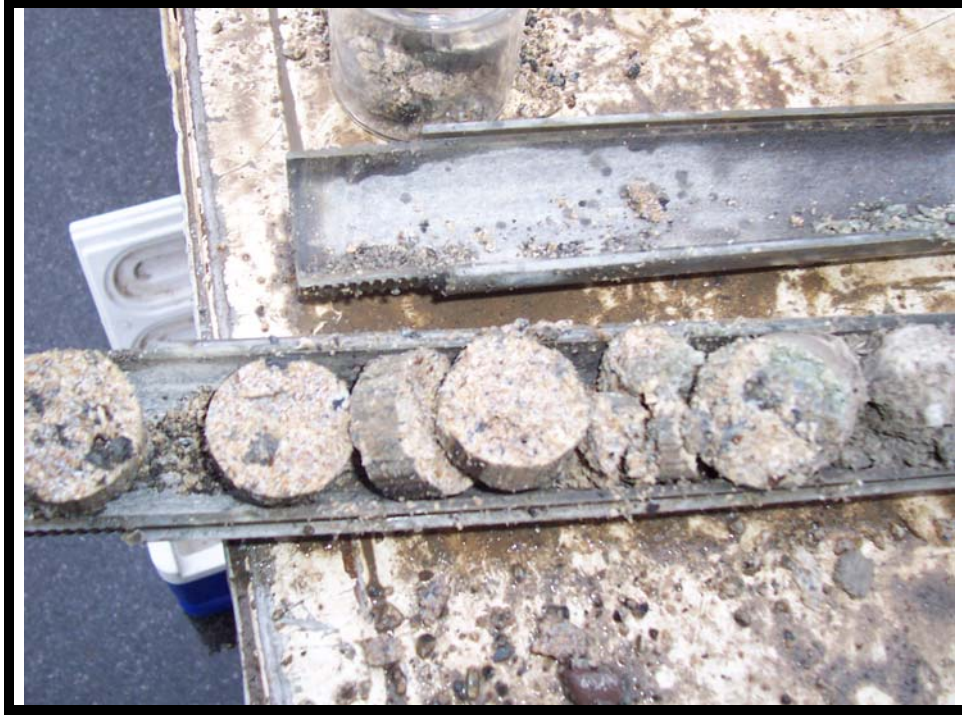
View of partially fused ash with trace gray and black metallic slag encountered in fill material collected from boring BS-37 [8.0' to 8.4'].
